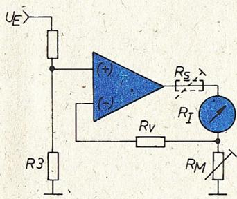
$$R_3 \approx R_v + R_m \parallel (R_f + R_s)$$
