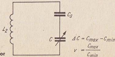
$$\Delta C_{ges} = \frac{C_{max} \cdot C_s}{C_{max} + C_s} - \frac{C_{min} \cdot C_s}{C_{min} + C_s}$$
