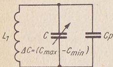
$$\Delta C_{ges} = (C_{max} + C_p) - (C_{min} + C_p) = konst. = \Delta C$$
